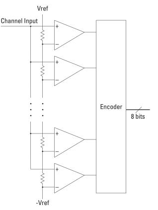
**Block Diagram of an ADC**
