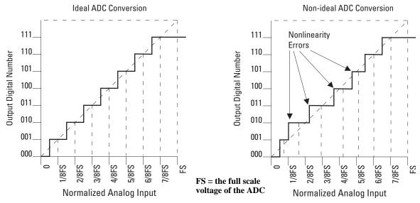
ADC Non-linearity Errors for a 3-bit ADC
